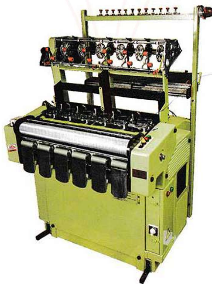
6/80 High speed needle loom
